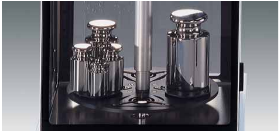
Comparison of mass standards as groups of weights using the CCE1000S-L
