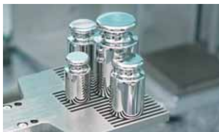
Comb-type weight grabber with 4 weights
